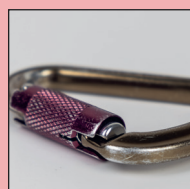
Locking mechanism defective
